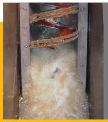
The turbulent zone of influence created by the optional patented TurboWash™ agitator loosens and emulsifies the organic BOD material on screenings.
